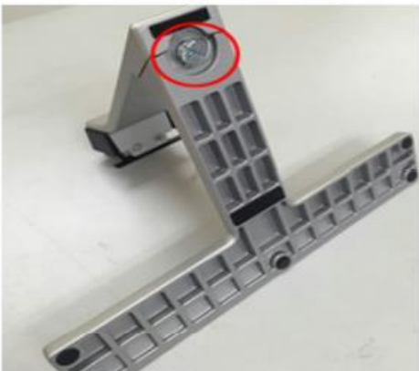
Step11. Unscrew two screws and separate base & neck assembly
