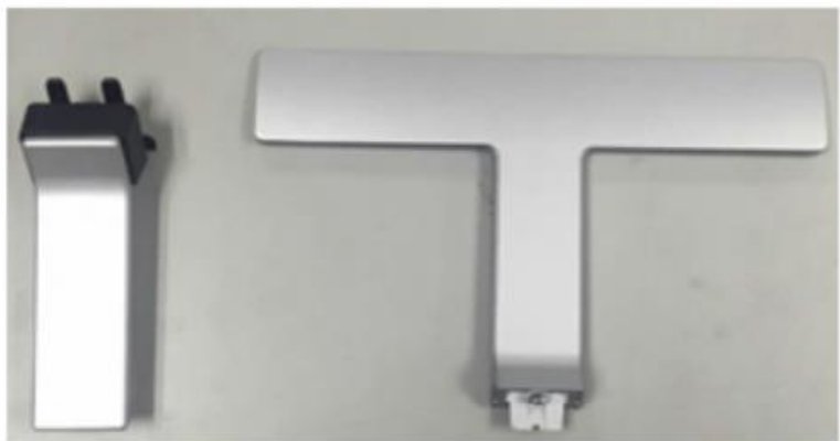
Step11. Unscrew two screws and separate base & neck assembly
